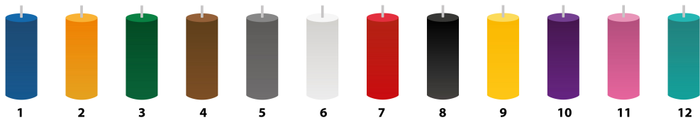
Colour coding (as per TIA-598-C)
