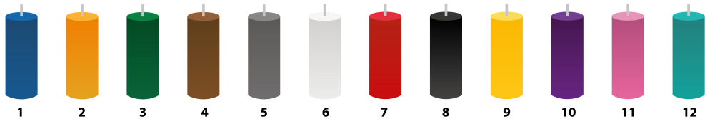
Colour coding (as per TIA-598-C)
