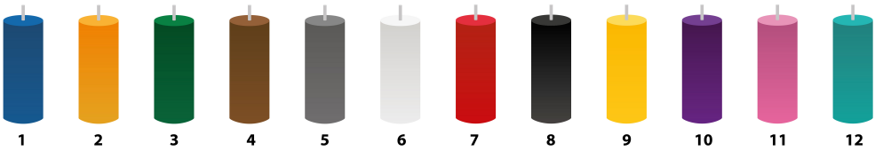
Colour coding (as per TIA-598-C)
