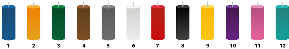
Colour coding (as per TIA-598-C)
