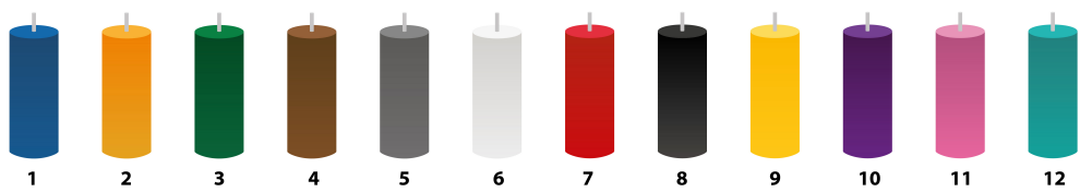
Colour coding (as per TIA-598-C)
