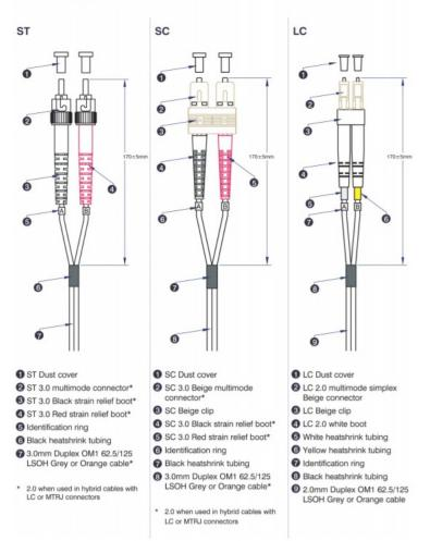
Excel Enbeam OM1 Fibre Optic Patch Lead LC-LC Multimode 62.5/125 DX LS0H Grey 2 m
