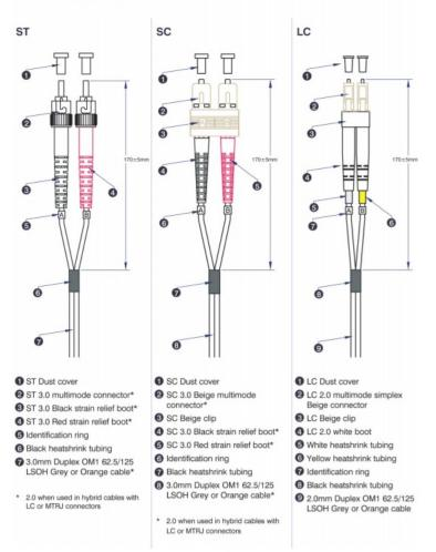
Excel Enbeam OM1 Fibre Optic Patch Lead LC-LC Multimode 62.5/125 DX LS0H Grey 5 m
