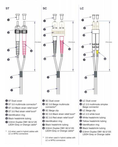
Excel Enbeam OM2 Fibre Optic Patch Lead ST-ST Multimode 50/125 DX LS0H Orange 10 m
