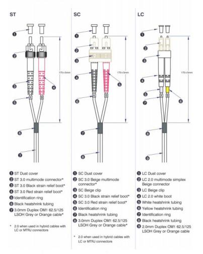
Excel Enbeam OM2 Fibre Optic Patch Lead ST-SC Multimode 50/125 DX LS0H Orange 1 m
