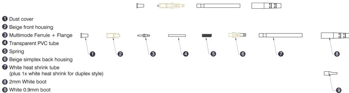
Note: Duplex version consists of 2 of each component shown plus a beige joining clip.
