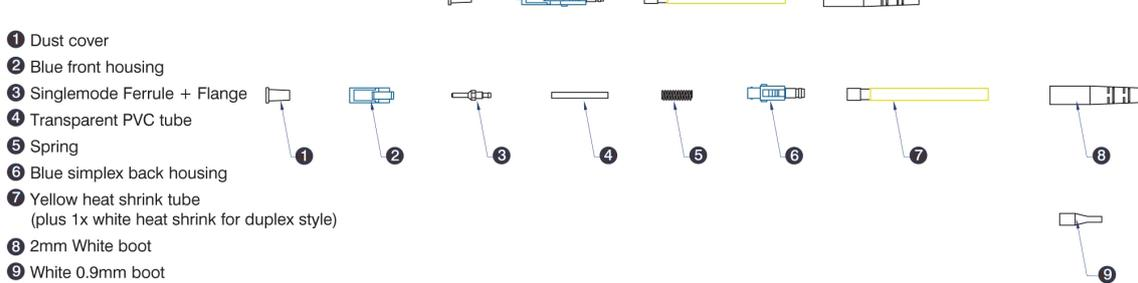
Note: Duplex version consists of 2 of each component shown plus a blue joining clip.
