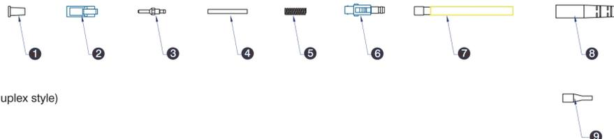
Note: Duplex version consists of 2 of each component shown plus a blue joining clip.
