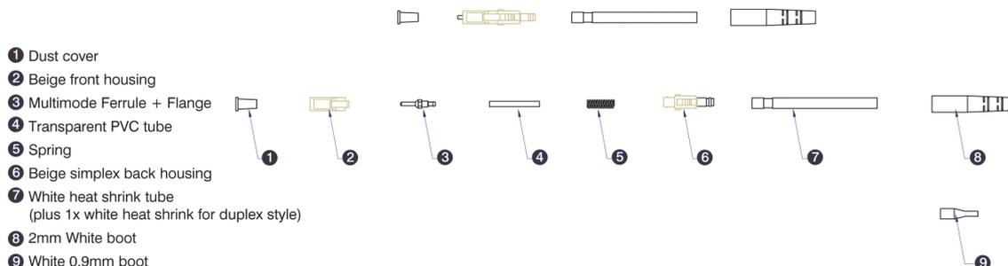
Note: Duplex version consists of 2 of each component shown plus a beige jointing clip.
