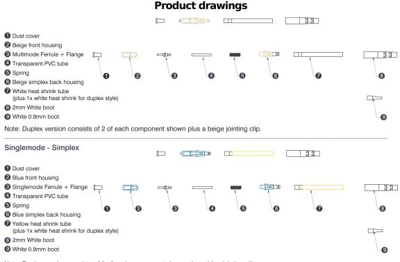
Note: Duplex version consists of 2 of each component shown plus a blue jointing clip.
