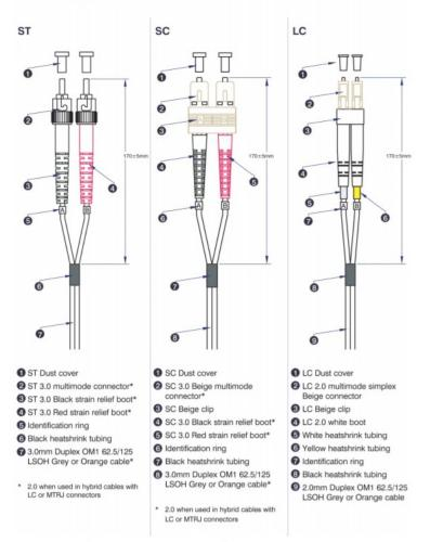
Excel Enbeam OM1 Fibre Optic Patch Lead SC-SC Multimode 62.5/125 DX LS0H Grey 2 m
