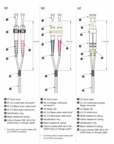
Excel Enbeam OM1 Fibre Optic Patch Lead SC-SC Multimode 62.5/125 DX LS0H Grey 5 m
