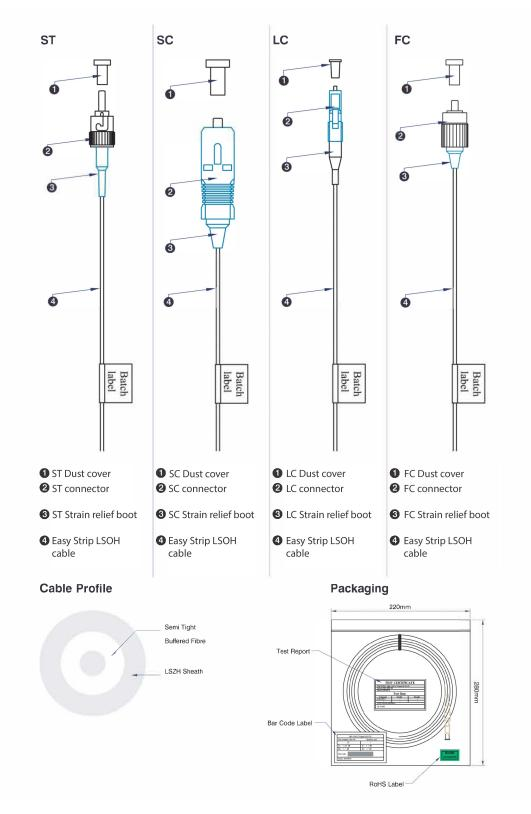
Excel Enbeam Fibre Pigtail OS2 9/125 LC/UPC Easy Strip 12-Colour Pack (TIA 598) 2 m
