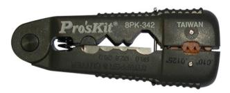
X Tri-hole tool removes 2-3mm tight jacket, 900μm secondary buffer and 250μm primary coatings
