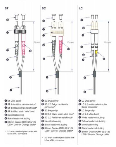
Excel Enbeam OM1 Fibre Optic Patch Lead LC-ST Multimode 62.5/125 DX LS0H Grey 0.5 m
