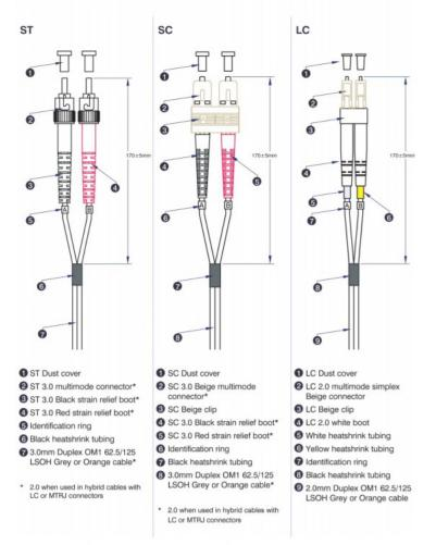
Excel Enbeam OM2 Fibre Optic Patch Lead SC-SC Multimode 50/125 DX LS0H Orange 0.5 m
