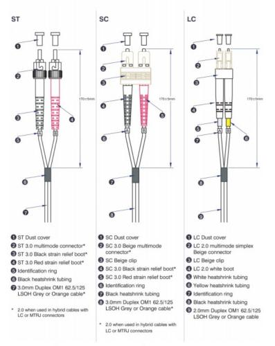
Excel Enbeam OM1 Fibre Optic Patch Lead ST-ST Multimode 62.5/125 DX LS0H Grey 0.5 m
