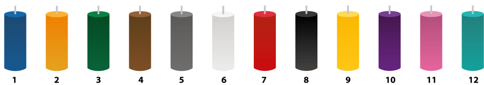
Colour coding (as per TIA-598-C)
