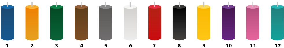
Colour coding (as per TIA-598-C)
