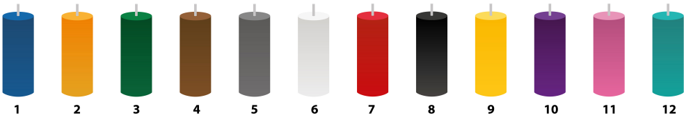
Colour coding (as per TIA-598-C)
