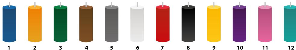
For fibre core counts above 12 the colour sequence is repeated with the addition of a mark every 70mm for cores 13-24 and two marks for 25-36 and so on.
