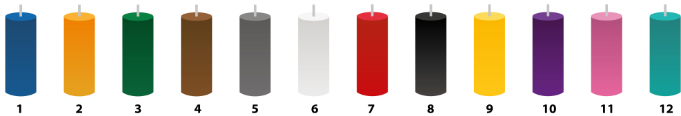
Colour coding (as per TIA-598-C)
