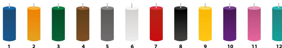
For fibre core counts above 12 the colour sequence is repeated with the addition of a mark every 70mm for cores 13-24 and two marks for 25-36 and so on.
