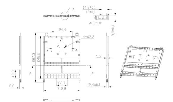
Excel Enbeam High Density 12 Port 24 Fibre LC OS2 Cassette Loaded with Duplex Adaptors
