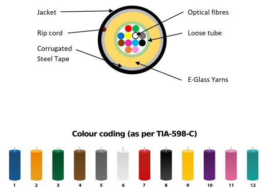
For fibre core counts above 12 the colour sequence is repeated with the addition of a mark every 70mm for cores 13-24 and two marks for 25-36 and so on.
