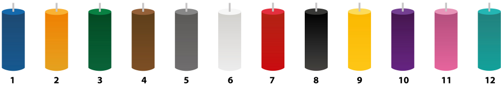
Colour coding (as per TIA-598-C)
