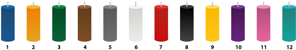
Colour coding (as per TIA-598-C)
