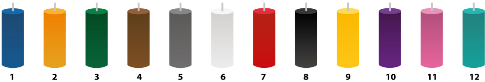
Colour coding (as per TIA-598-C)
