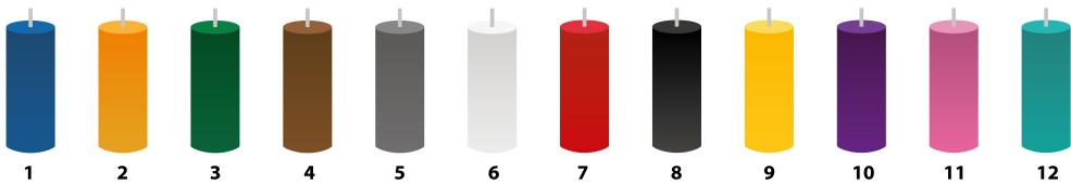
Colour coding (as per TIA-598-C)
