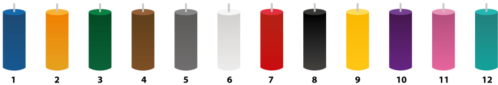
Colour coding (as per TIA-598-C)
