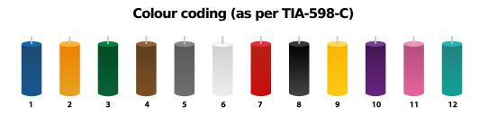
For fibre core counts above 12 the colour sequence is repeated with the addition of a mark every 70mm for cores 13-24 and two marks for 25-36 and so on.
