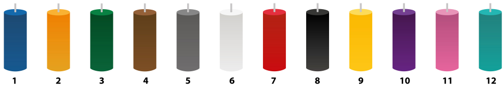
Colour coding (as per TIA-598-C)
