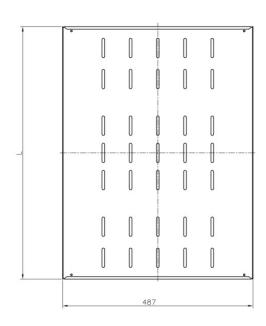
Material: SPCC Cold Rolled Steel; Thickness: 1.2mm
