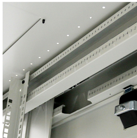
Quick slam latches and position No.s
