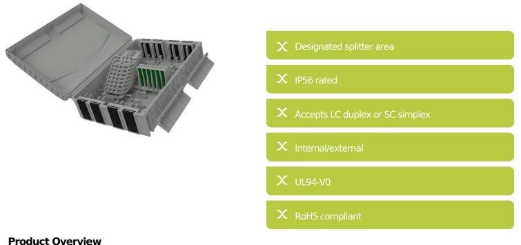
The Encasa range of fibre distribution points have been designed to fit within the FTTx network. These enclosures can be aerial or wall mounted. Made from 100% virgin UL94-V0 rated material, UV stable and are IP56 rated, allowing them to be used in both internal and external applications. This Encasa fibre distribution point accommodates 96 fibres (using LC connections) or 48 fibres (using SC connections).
