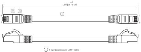
(2) RJ45 connector with 50 $\mu$ m gold plated staggered pins
