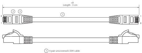
2 RJ45 connector with 50µm gold plated staggered pins
